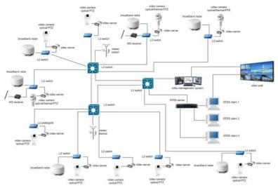
Figure 3: Coastline Surveillance and Tracking Security System – STSS-Carchitecture [2]
