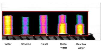
Figure 2: Cargo Inspection – discrimination of petroleum products
